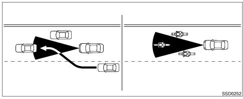
The detection zone of the ICC sensor is limited. A vehicle ahead must be in the detection zone for the vehicle-to-vehicle distance detection mode to maintain the selected distance from the vehicle ahead.
