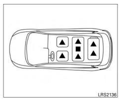
The illustration shows the seating positions equipped with head restraints. The third row head restraints are removable but not adjustable.
