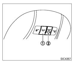
When the ON switch (1) is pressed, the footwell lights, step lights, map lights and rear personal lights will automatically turn on and stay on for a period of time when:
