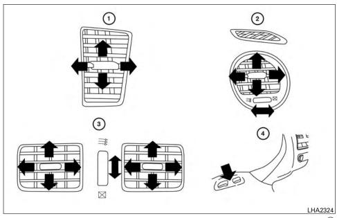
Adjust air flow direction for the driver's and passenger's side vents (1), center vents (2), and rear vents (3) by moving the vent slide and/or vent assemblies.
