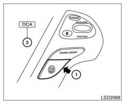
To turn on the DCA system, push the dynamic driver assistance switch ① on the steering wheel after starting the engine. The Distance Control Assist (DCA) system switch indicator light ② in the vehicle information display will illuminate. Push the dynamic driver assistance switch again to turn off the DCA system. The Distance Control Assist (DCA) system switch indicator light will turn off.
