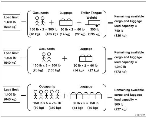
Steps for determining correct load limit
