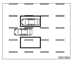
If the BSI system is on and your vehicle approaches the lane marker while another vehicle is in the detection zone, the Blind spot warning indicator light flashes and a chime will sound three times. Then, the BSI system slightly applies the brakes on one side to help return the vehicle back to the center of the driving lane.
