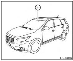
The Lane Departure Warning (LDW) system/ Lane Departure Prevention (LDP) system will operate when the vehicle is driven at speeds of approximately 45 MPH (70 km/h) and above, and when it is traveling close to either the left or the right of a traveling lane.
