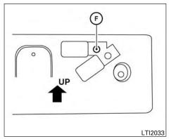
Mark the center of the hole (F) on both sides with a felt-tip pen. Remove the bracket from the bumper, and then open 0.79 in (20 mm) diameter holes on the bumper using the marks (F) as a center.
