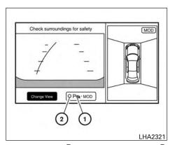
When the switch ① is selected, the indicator ② will turn off and the sonar will be turned off temporarily. The MOD system will also be turned off at the same time. When the switch is selected again, the indicator will turn on and the sonar will turn back on.
