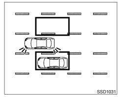
If the driver activates the turn signal, then the system chimes a sound (twice) and the Blind spot warning indicator light flashes.
