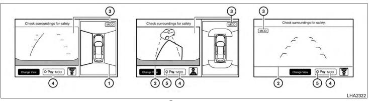
If the MOD system detects the moving objects surrounding the vehicle, the yellow frame will be displayed on the camera image and a chime sounds.
