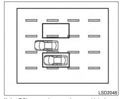
If the BSI system is on and your vehicle is approaching a lane marker, the system chimes a sound (three times), and the Blind spot warning indicator light flashes. Then the BSI system slightly applies the brakes on one side to help return the vehicle back to the center of the driving lane.
