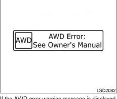
If the AWD error warning message is displayed, there may be a malfunction in the Intelligent AWD system. Reduce vehicle speed and have your vehicle checked by an INFINITI retailer as soon as possible.
