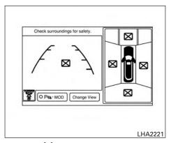
When the "[X]" icon is displayed on the screen. the camera image may be receiving temporary electronic disturbances from surrounding devices. This will not hinder normal driving operation but the system should be inspected by an INFINITI retailer if it occurs frequently.
