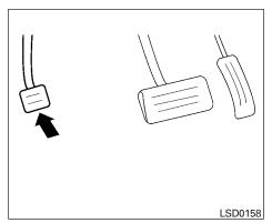
To engage: Firmly depress the parking brake.
