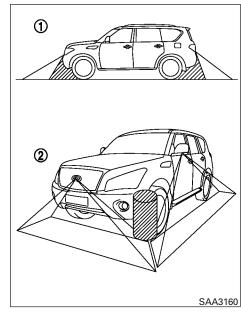
There are some areas where the system will not show objects. When in the front or rearview display, an object below the bumper or on the ground may not be viewed (1). When in the bird-eye view, a tall object near the seam of the camera viewing areas will not appear in the monitor (2).
