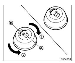
The climate controlled seat warms up or cools down the front seat by blowing warm or cool air from the surface of the seat. The climate control switch is located on the center console.
