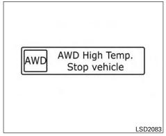
The AWD high temperature message may be displayed while trying to free a stuck vehicle due to increased oil temperature. The driving mode may change to two-wheel drive. If this message is displayed, stop the vehicle with the engine idling, as soon as it is safe to do so. Then if the message turns off, you can continue driving.
