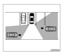
A red frame will appear in the center display, the system will chime 3 times and the brakes will be applied for a moment, if an approaching vehicle is detected when your vehicle is backing up. After the automatic brake application, the driver must depress the brake pedal to maintain brake pressure.
