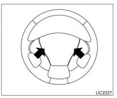
To sound the horn, push near the horn icon of the steering wheel.
