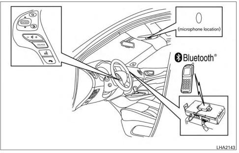
Your INFINITI is equipped with the Bluetooth® Hands-Free Phone System. If you have a compatible Bluetooth® enabled cellular phone, you can set up the wireless connection between your cellular phone and the in-vehicle phone module. With Bluetooth® wireless technology, you can
