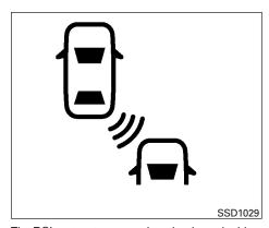
The BSI system turns on when the dynamic driver assistance switch on the steering wheel is pushed when the "Blind Spot Intervention" is enabled in the settings menu on the meter display. The BSI ON indicator light (green) on the instrument panel illuminates when the BSI system is turned on.
