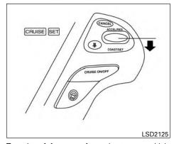
To set cruising speed, accelerate your vehicle to the desired speed, push the COAST/SET switch and release it. (Vehicle ahead detection indicator, set distance indicator and set vehicle speed indicator (B) will come on.) Take your foot off the accelerator pedal. Your vehicle will maintain the set speed.
