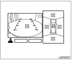
If the radar detects an approaching vehicle from the side, the system chimes a sound (single beep), the Blind spot warning indicator light on the side the approaching vehicle flashes and a yellow rectangular frame appears in the display.
