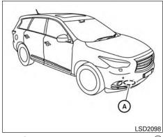
The FCW system uses the distance sensor (A) located behind the front bumper to measure the distance to the vehicle ahead. When the system judges that your vehicle is getting close to the vehicle ahead in the travel lane, the vehicle ahead detection indicator light on the instrument panel blinks and a warning chime sounds.
