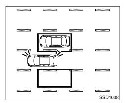
If the driver activates the turn signal, then the Blind spot warning indicator light flashes and a chime will sound twice.
