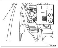
Check the fluid level in the reservoir.
