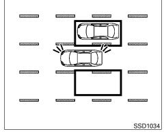
If the driver activates the turn signal while another vehicle is in the detection zone, then the system chimes a sound (twice) and the Blind spot warning indicator light flashes.
