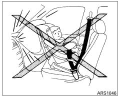
Even with the INFINITI Advanced Air Bag System, never install a rear-facing child restraint in the front seat. An inflating front air bag could seriously injure or kill your child. See "Child restraints" earlier in this section for details.
