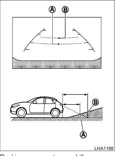
the hill is the place (B). Note that any object on the hill is further than it appears on the monitor.
