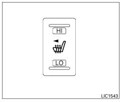
The rear seats are warmed by built-in heaters. The switches are located on the rear of the front center console and can be operated independently of each other.
