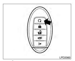
The **Q** button will be on the INFINITI Intelligent Key if the vehicle has remote engine start. This feature allows the engine to start from outside the vehicle.
