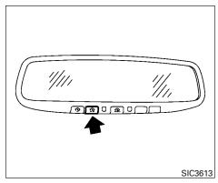
3. Using both hands, simultaneously press and hold both the HomeLink® button you want to program and the hand-held transmitter button.
