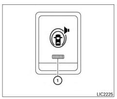
The warning systems switch is used to turn on and off the warning systems (Forward Collision Warning (FCW), Lane Departure Warning (LDW) and Blind Spot Warning (BSW) systems) that are activated using the settings menu on the center display.
