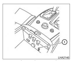
Front AUX (auxiliary) input jacks (inside center console)
