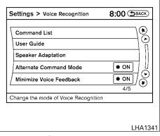
Alternate Command Mode is activated and the setting menu is expanded to include the Alternate Command Mode options. See "Settings menu" in this section for an explanation of the options.
